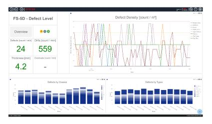
The overview of defects identified by types and their classes using a flat glass inspection system as an example allows conclusions to be drawn on the system's condition.
