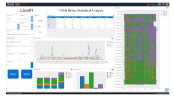
Statistical defect analysis using an inspection system for solar glass production as an example – including defect distribution and/or type clustering of the solar glass ribbon.
